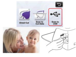
If you want to use the image from a hard-to-replace photo, use the Scan to USB function to copy the photo and save it as data. You can then print out and cut the saved photo data instead of the original photo. Function: Scan to USB
